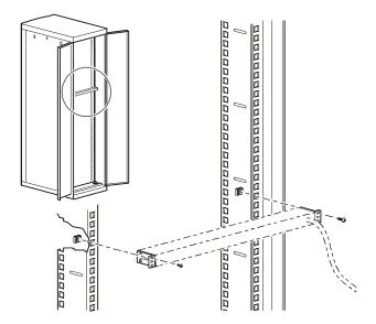
Vertical mounting (any standard EIA-310 rack or enclosure) Install the PDU in a NetShelter or any standard 19-inch EIA-310 rack or enclosure, using the mounting brackets (provided).
