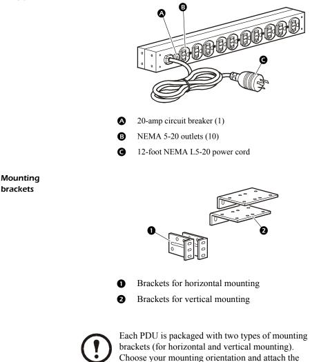
appropriate brackets to the PDU for installation.
