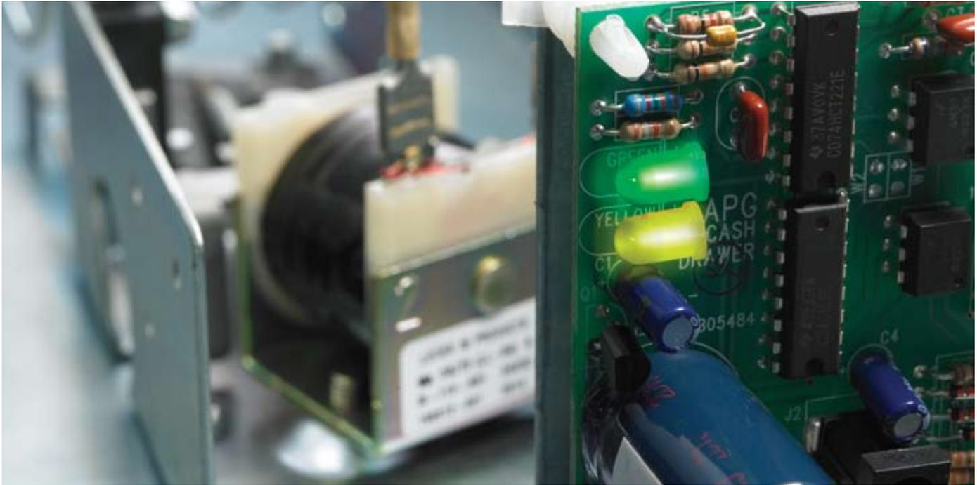
All APG board level products feature accessible diagnostic lights, making set-up and trouble-shooting easy.
