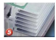
The Black Max's **two large custom extruded heat sinks** add 8 lbs. to the total amplifier weight. The half-inch thick extrusion base provides exceptional heat transfer from the output devices, lowering the junction temperatures and extending their life.
