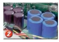
**74,600 µf of capacitance** filters the 110V DC power supply rails creating enormous energy reserve for low distortion, full power bass. The capacitor's 105° F temperature rating ensures long life even under the most harsh conditions.
