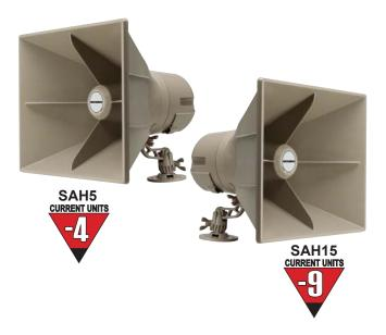
**Description** The SAH5 and SAH15 powered horn loudspeakers employ digital switching amplifier technology resulting in low DC current draw and low heat dissipation. This means fewer power supplies, longer cable runs, and the capacity to work at higher ambient temperatures when compared to conventional analog self-amplified horn speakers.
