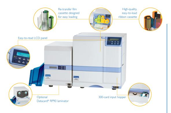
The Datacard® RP90 card printer uses unique re-transfer printing technology to deliver exceptional, full coverage on a wide range of non-PVC cards, including contact and contactless smart cards.
