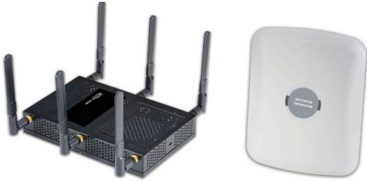
*Altitude™ 4610 and 4620 are high-performance, dual-radio access points that enable secure and cost-effective deployment and operation of 802.11n based Enterprise wireless LANs.*
