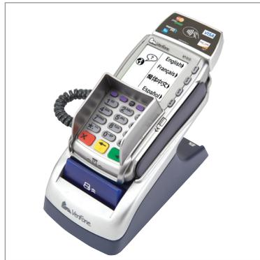
The modularity of the V<sup>x</sup> 810 allows for a variety of options, including contactless payment, a base unit with a printer and modem to make it a complete payment device, and a privacy shield for added consumer protection.
